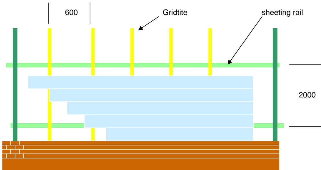
The standard Gridtite bar / bar push fit joint is **not** designed to carry cladding loads applied *along* the bar as is found in upright fixing. Inserting a fastener into the pre-punched holes in the socket joint will lock both bars together and will help to transmit loads.
