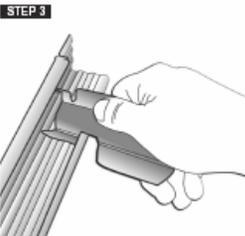
*3 Rotate the bracket away from you to hook the smaller tab in place under the bar edge*
