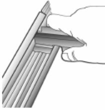
5. Finally, rotate the bracket round to approx 90° to lock it in place
