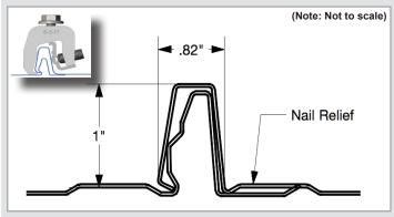
(NOTE: Seams that exceed maximum allowance at the widest part of the seam will require hand crimping to allow the clamp to fit).
