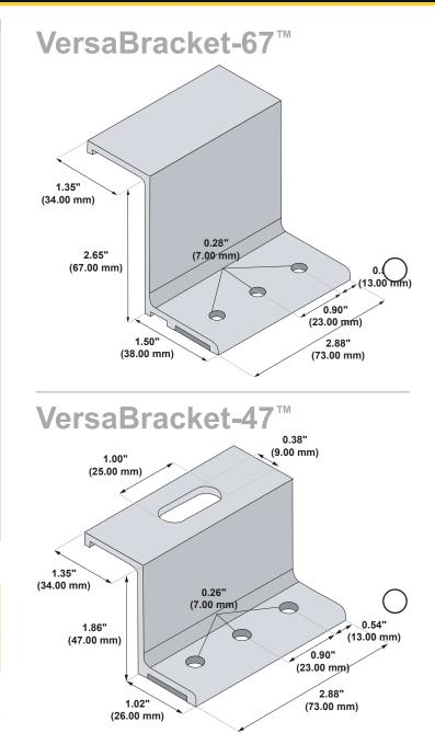
3 holes are provided for versatility. Some installations require only 2 fasteners. See the load table on the S-51 website and the installation instructions for more details.
