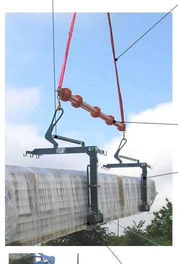
Forks locate in wooden pallets below packs and prevent any panel damage
