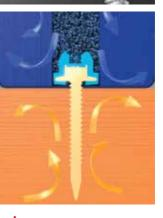
Hot box tests and thermal activity recording has repeatedly shown that the composition of the Opticore head provides better thermal retention values over metal
