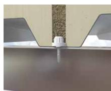
Opticore is EJOT's unique and patented integral nylon head, designed to encapsulate fasteners from our high performance Self-Drilling range. Opticore is engineered to provide a dual drive fastening system that enables rapid self-coring of membrane faced insulation panels, and a secure fix into hot and cold rolled steel, and
