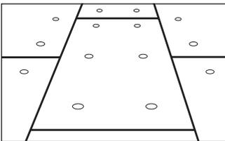
**Lay insulation** over substrate. Place plates in pattern specified by roofing system manufacturer.
