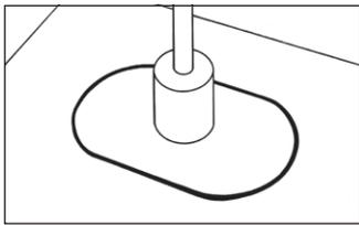
**Remove RhinoBond tool** after the cycle ends and immediately set a magnetic heat sink directly onto the center of the plate.
