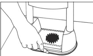
**While the RhinoBond is activated (welding), trace around the base** of the tool with a grease pencil. This will help you judge your accuracy in centering the coil over the plate.
