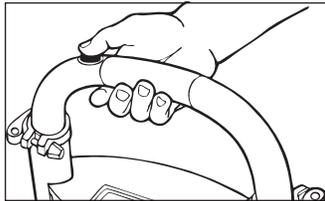
Center the calibrated RhinoBond tool over the first plate in pattern and activate the weld.
