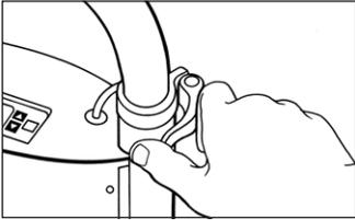
Adjust the handle height, if desired, loosening clamp by twisting to the left, by releasing handle clamps and gently pulling or pushing handle to desired position.
