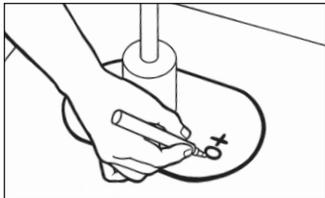
**Mark the energy setting** next to the plate position with a grease pencil.
