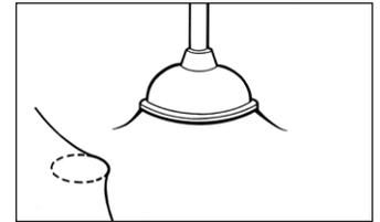
To determine if a weld has been made, place the plunger next to a welded plate and create enough suction to lift the membrane. A weld will create the membrane as shown. If the assembly is not welded, the membrane will lift up from the plate.
