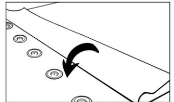
**Place 5 plates** on a sample of your insulation, 10 inches (250mm) apart. (Do **NOT** use screws.) Lay a sample of your membrane over the plates.
