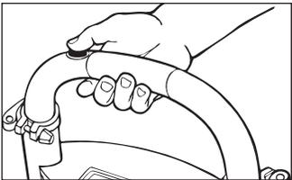
**Activate the weld** using the activation button on the handle.
