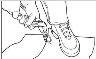
**Use pliers to peel each plate off** of the membrane.
