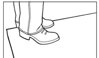
**Locate each plate** by rubbing the membrane with the sole of your shoe.
