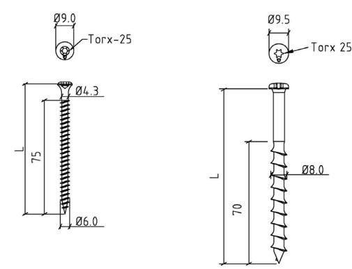
Fig. 23 LBS 6.0 screw for lightweight concrete, concrete and wooden substrates
