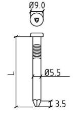
Fig. 19 BNRF 5.5 Stainless concrete nail
