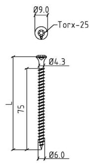
Fig. 39 LBS 6.0 Screw for light weight concrete, concrete and wooden substrates
