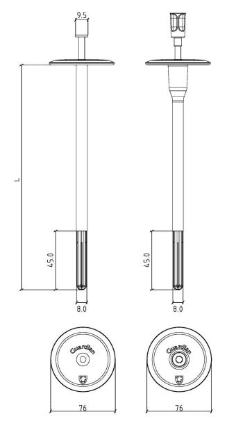
Fig. 22 CPN-8 Concrete plug CP-8 Concrete plug with energy bridge stop (also usable with SP-70-CP)
