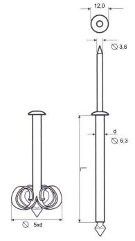
Fig. 36 GPR 6.3 Peel Rivet
