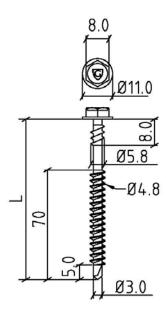
Fig. 30 DBT(A) 4.8 Screw for fixing in steel sheets (usable with automatic setting tool)
