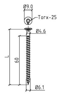
Fig. 40 HD 6.1 Screw for light weight concrete, concrete and wooden substrates
