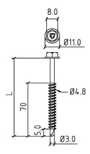
Fig. 31 DB(A) 4.8 Screw for fixing in steel sheets (usable with automatic setting tool)
