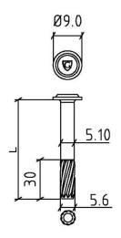
Fig. 18 BN 5.6 Concrete nail
