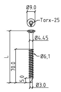
Fig. 34 BS 6.1 Screw for fixing in steel sheets
