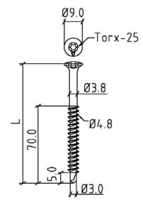
Fig. 27 BS 4.8 Screw for fixing in steel sheets
