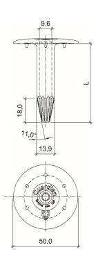
Fig. 3 Tube washer RBS 50 with six barbs
