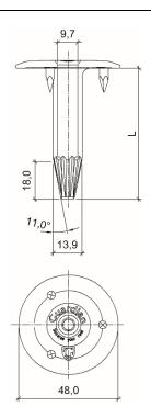
Fig. 2 Tube washer RB 48 with three barbs
