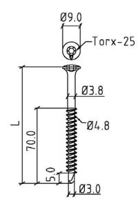
Fig. 29 BSRF 4.8 Stainless screw for fixing in steel sheets
