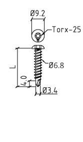
Fig. 35 BS 6.8 Screw for fixing in thin steel sheets
