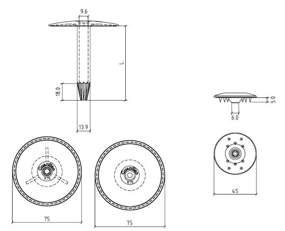
Fig. 5 Tube washer R-75 Tube washer HR-75 with hexagonal internal tube shape (used together with ACS 6.1)
