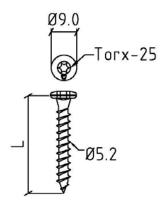
Fig. 37 TS 5.2 Screw for fixing in wood
