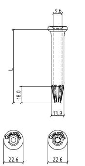
Fig. 16 GWT tube for GWSP(\*)-80-F4E (Polyamide) CT tube for STBT (Polypropylene)
