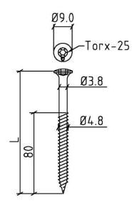
Fig. 26 PS 4.8 Screw for fixing in steel sheets
