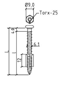
Fig. 21 ACS 6.1 Adjustable concrete screw (used together with tube washer HR versions)
