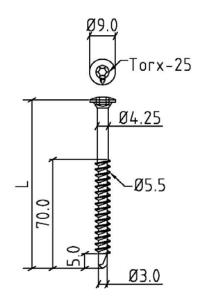
Fig. 33 BS 5.5 Screw for fixing in steel sheets
