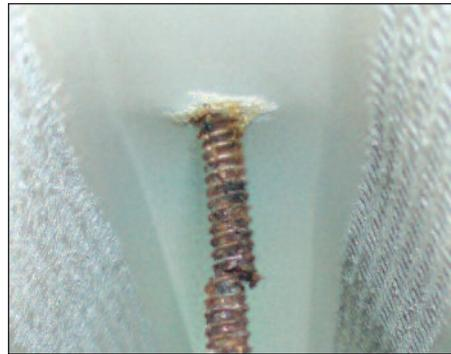
Minimising the potential for bimetallic corrosion and natural corrosion of fasteners is generally aided by the addition of protective coatings. These coatings can range from a passivated zinc coating applied to austenitic stainless steel bi-met fasteners, through to a combination of zinc and organic corrosion-resistant coating applied to carbon steel fasteners.
