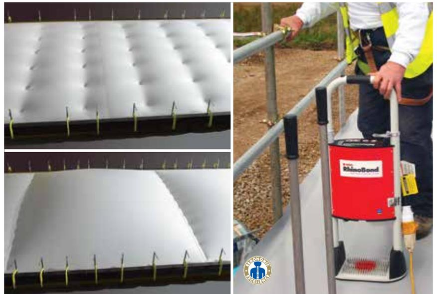
*The RhinoBond welded membrane spreads the wind load evenly across the roof (top) as opposed to the traditional in-seam fixing method (bottom).*
