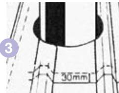
3 Mark the outline of the soaker on the roof then remove it. Mark a lap allowance of 30mm (inside the original mark). Now determine where soaker sides will finish.
