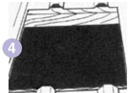
4 Remove all roof inside the 30mm line. Trim off any sharp or uneven edges. Timber supports must be installed to support the roof where the ribs have been removed. (Pipe removed for drawing clarity)
