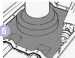
6 Fix self tapping and self-sealing screws to the middle front and middle back of the soaker and fix progressively towards the edge.
