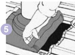
5 Replace the soaker in position and apply silicone sealant to the roof while holding up the edge of the flashing.
